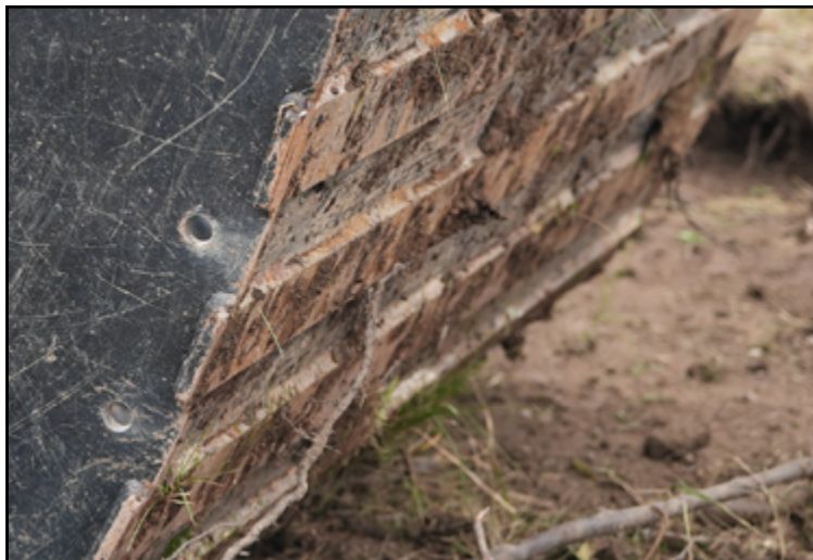
Figure 3: Wear plates reinforce the back skin
